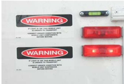
Transport Warning Lights
