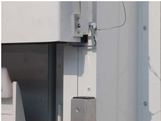
Figure 39: Right Side Slide-out, Outside Canopy-Locking Pin (Installed)
