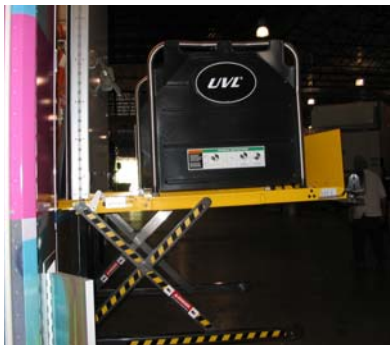
Platform lift carriage in the raised position to the mobile unit floor level
