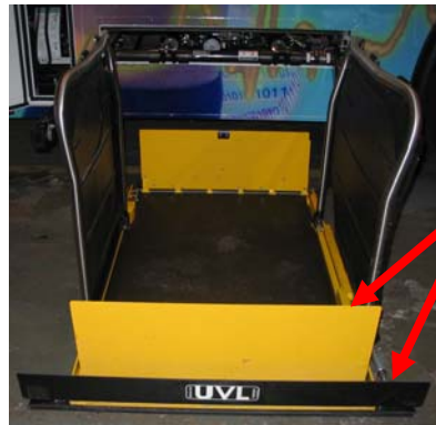
Folded handrails in the vertical and secured position. The outer Barriers will deploy automatically when the platform makes contact with the ground.
