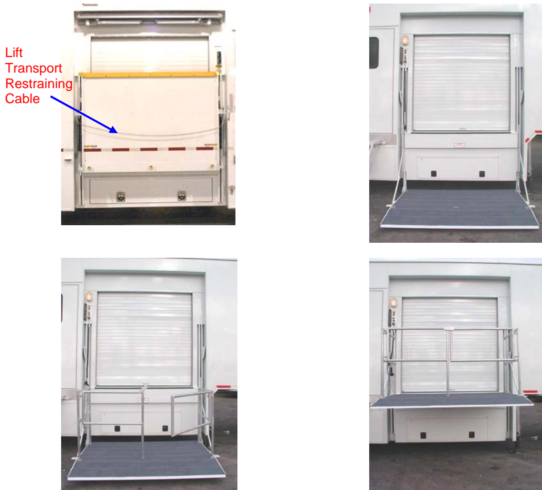
Figure 36: Platform Lift Progression
